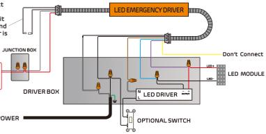
After installation is completed, join the LED emergency driver's connector and apply AC power
