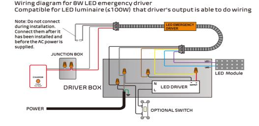
Wiring diagram for 8W LED emergency driver (Split Version) Compatible for LED luminaire (<100W) that driver's output is able to do wiring
